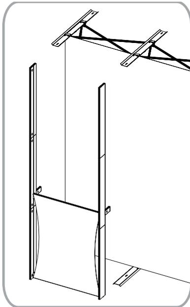
Lock extrusion frame onto top and bottom stabilizing feet, using fixed cam lock. With Allen Key tool, turn one quarter turn to lock into place.
