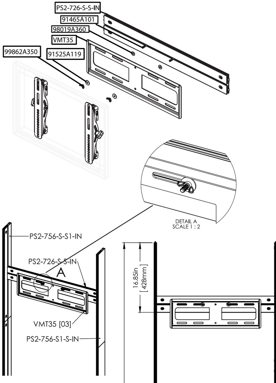
Attach shelf to frame. Lay shelf flat onto counter frame.
